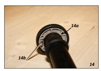
Both columns are initially equipped with 3/8-inch screws. On the long one only we can change it for a 1/4 inch screw. One must proceed as follows: using the large hex wrench, loosen the nut from the threaded rod (15), remove the rod by unscrewing it out (16), move the nut towards 1/4 inch end of the threaded rod (17) and the replace the whole to the desired height (18), finally tighten the nut.
